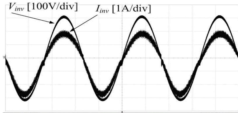
**Figure 3.** PV micro-inverter output current and voltage with +/- 2% chopping fraction.
