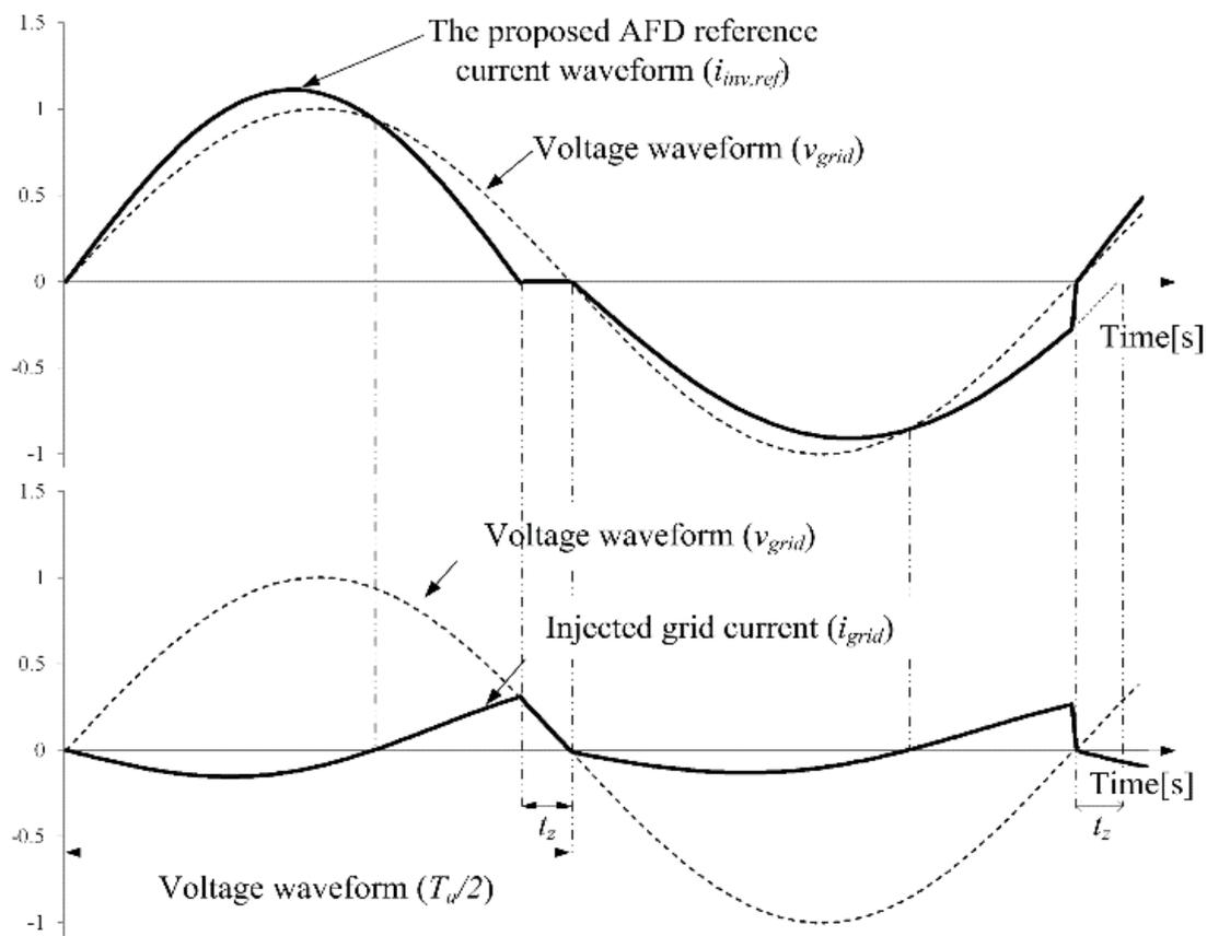
**Figure 1.** Operational waveforms for the proposed anti-islanding function.
