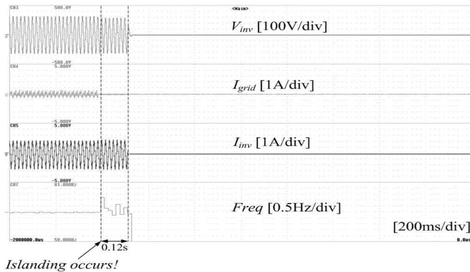
**Figure 4.** Anti-islanding test results for a single PV micro-inverter under a unity quality resonant load.
