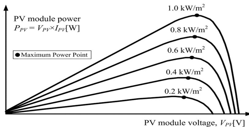
Figure 1. PV module electrical characteristics.
