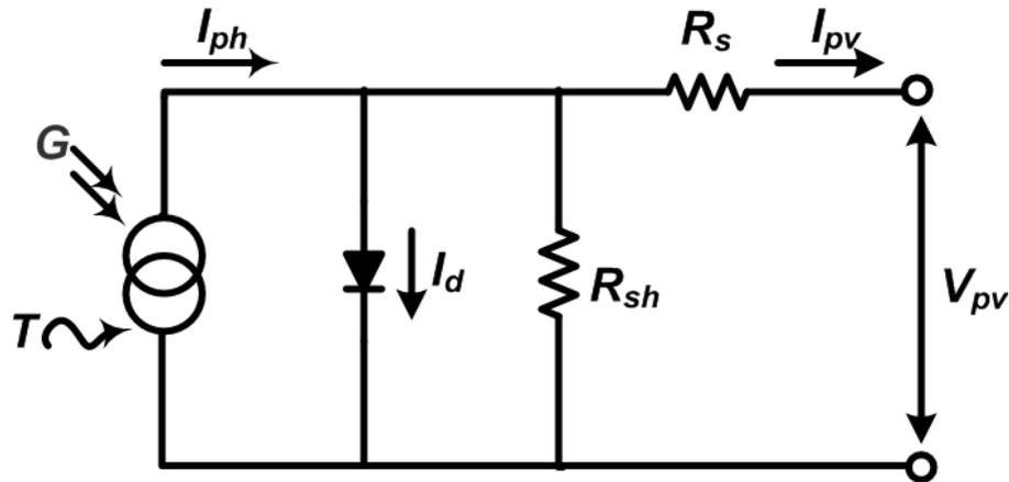
**Figure 2.** PV module electrical equivalent circuit.
