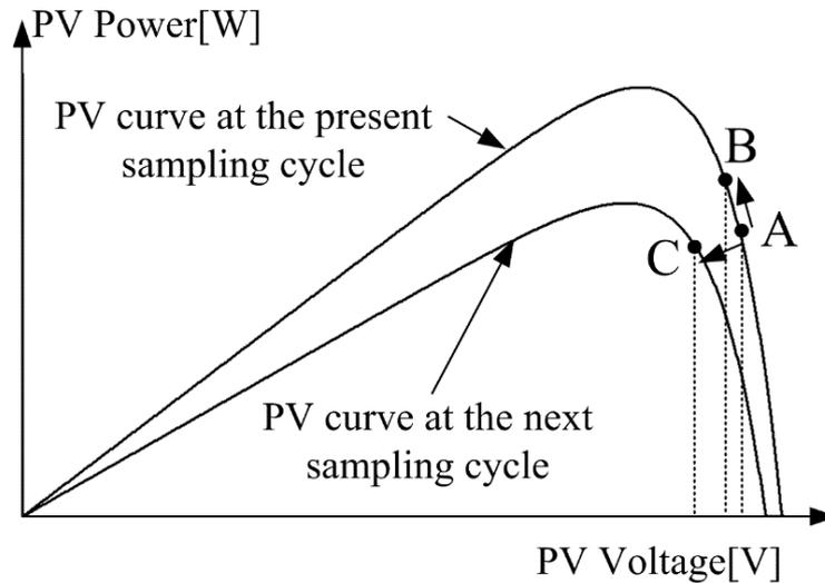
**Figure 4.** Power-voltage characteristics of PV module under rapidly changing irradiance environmental condition.
