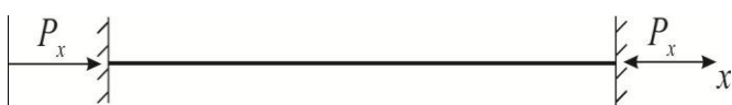
Figure 2: Moderately thick beam with fixed (clamped) ends at x = 0 , and x = l under compressive load
