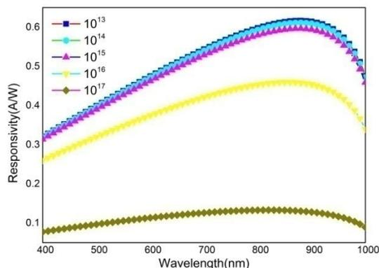
**Fig.11.** Responsivity variation with wavelength for different values of bulk defect density.
