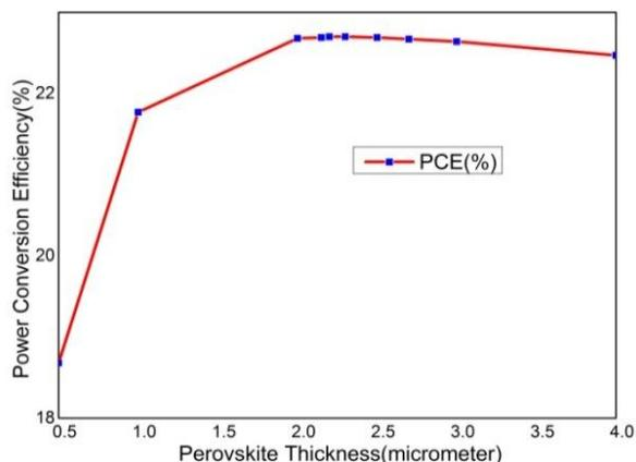
**Fig. 4(b).** Variation of Power Conversion Efficiency with perovskite absorber thickness.
