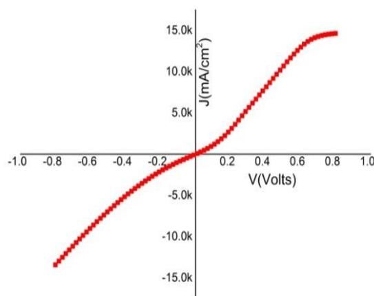
**Fig. 3.** J-V characteristic of Perovskite solar cell with Silver as back electrode.
