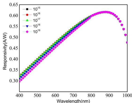
**Fig.12.** Responsivity variation with wavelength for different values of interface defect density.
