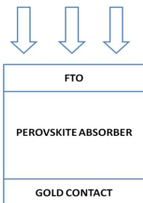
Fig.1(a). Perovskite device structure.
