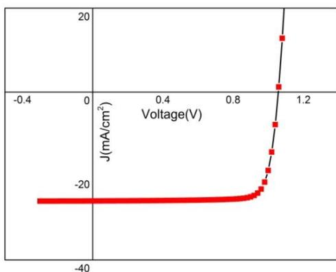
**Fig. 4. (a)** J-V curve for optimum perovskite absorber thickness of 2.3  $\mu\text{m}$ .
