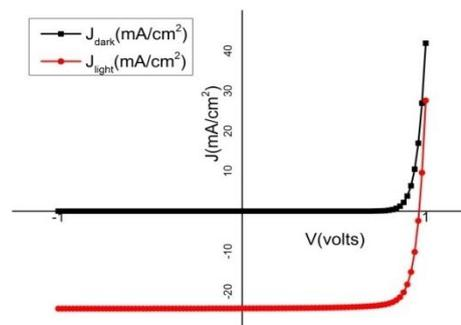
Fig. 2. J-V characteristic of Perovskite Solar Cell.
