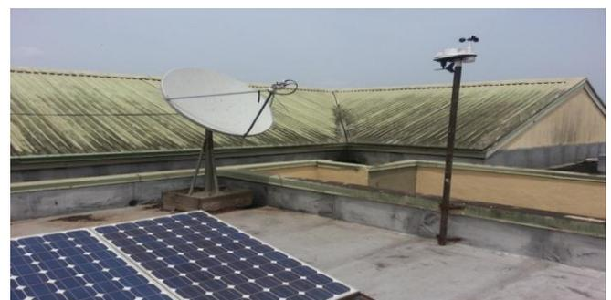
**Figure 2** The outdoor of the satellite dish pointing to space and the tipping bucket rain gauge
