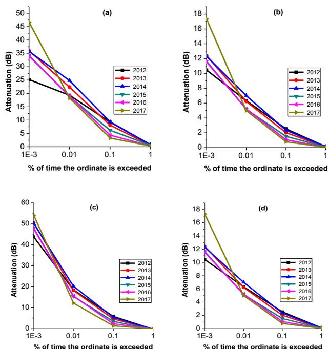
**Figure 4** The probability of exceedance curve computed for each rain attenuation model (a) Brazil Model and (b) Bryant Model (c) Crane Global Model and (d) Crane Two Components Model
