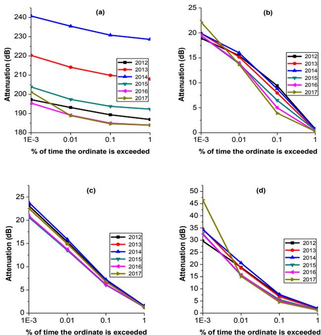
**Figure 5** The probability of exceedance curve computed for each rain attenuation model (a) EXCELL Model and (b) Garcia Model (c) ITU-R 618-13 Model and (d) Karasawa Model
