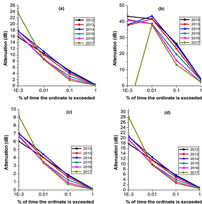
**Figure 6** The probability of exceedance curve computed for each rain attenuation model (a) Leitao-Watson Model and (b) Misme Waldteufel Model (c) SAM Model and (d) Svjatogor Model
