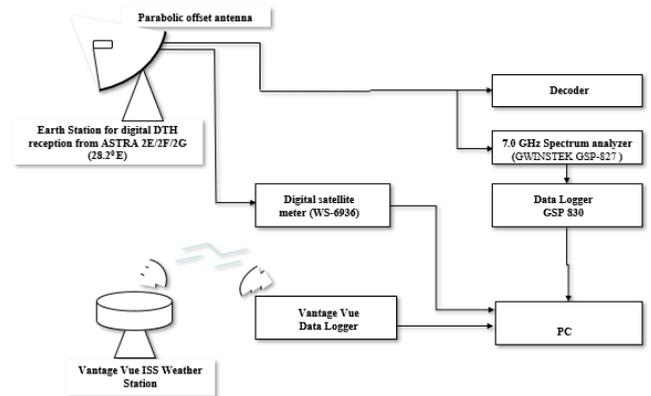
**Figure 1** Block diagram of the experimental setup at Covenant University, Ota
