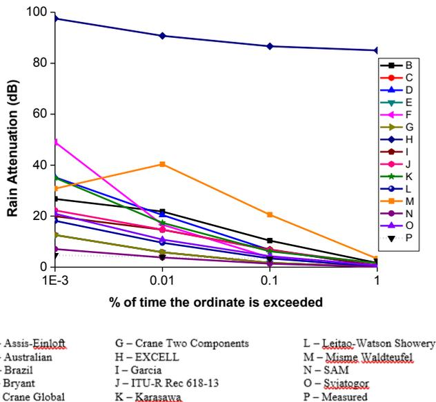
**Figure 7** Comparison between measured rain attenuation and existing predicted rain attenuation models at CU, Ota
