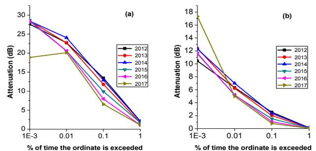
**Figure 3** The probability of exceedance curve computed for each rain attenuation model (a) Assis-Einloft Model and (b) Australian Model
