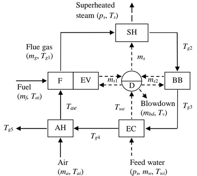
Fig. 2. Material flows in industrial boiler system
