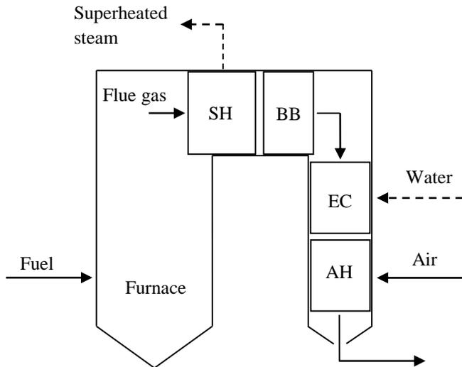
Fig. 1. Main components of industrial boiler
