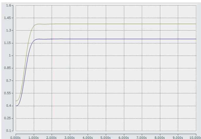
**Figure 15:** Simulation of the distributed system when the set-points are:  $y_{Maglev1}^{SP3} = 1.2[m]$  and  $y_{Maglev2}^{SP3} = 1.4[m]$
