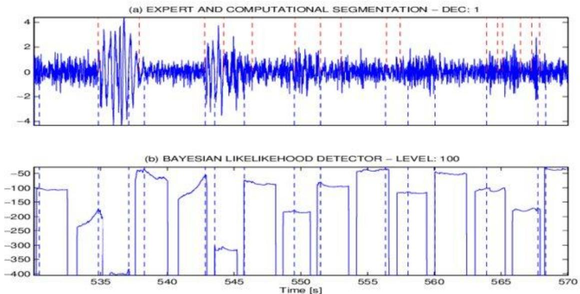
Fig. 3 Signal pattern presenting (a) segment by an experts (red) and by a Bayesian form of change-point detection (blue) and (b) a probability to detect change-points [29]
