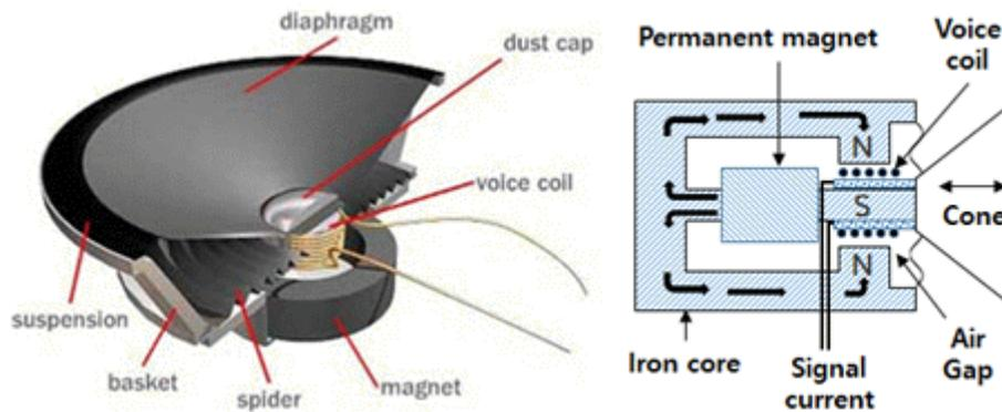
**Fig 2.** Structure of permanent-magnet type speaker [<http://www.audiocircuit.com/>][7]
