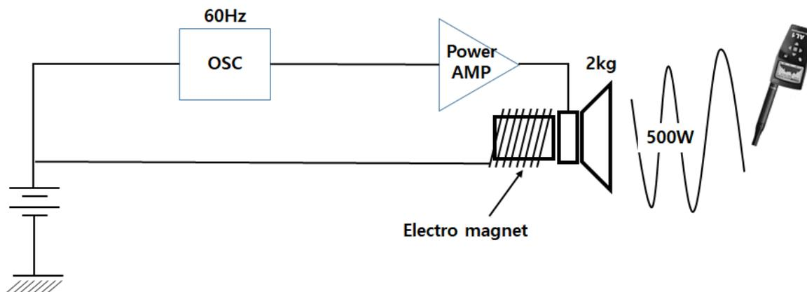
Fig 5. Output measurement using an improved electro-magnet type speaker
