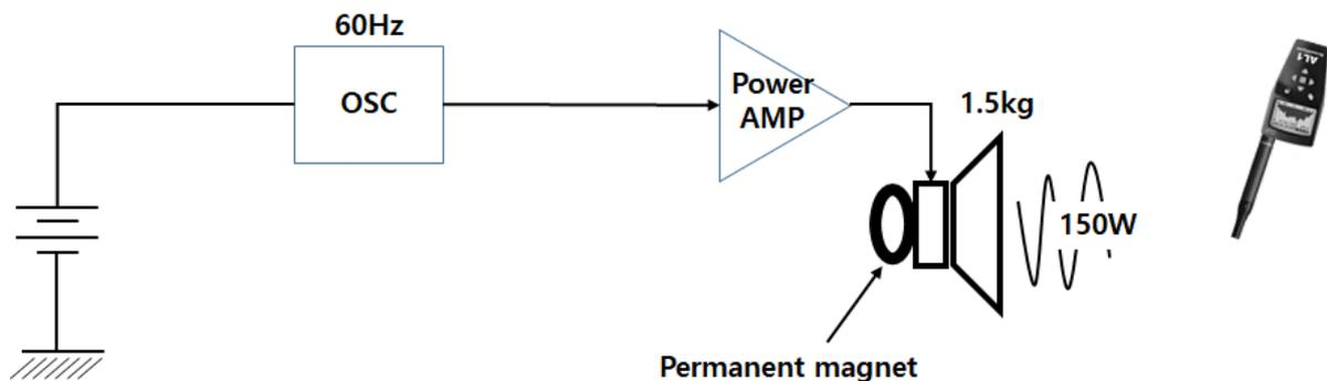
Fig 4. Output measurement using general permanent-magnet type speaker
