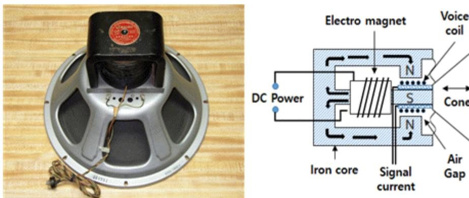
**Fig 3.** Structure of electro-magnet type speaker [<https://www.diyaudio.com/>][8]
