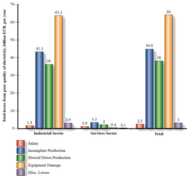
**Fig. 2.** Damage segmentation in terms of category consequences
