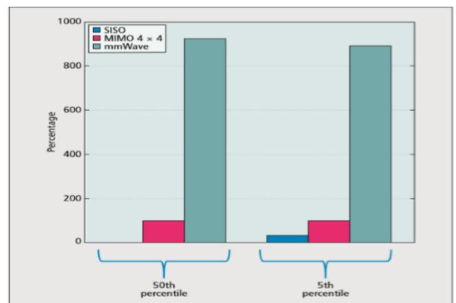
Figure 2. Cell data rate comparison between microwave systems using 50 MHz of bandwidth (single-user single-antenna and single-user MIMO) and a mmWave system with 500 MHz of bandwidth and a single user. [4].
