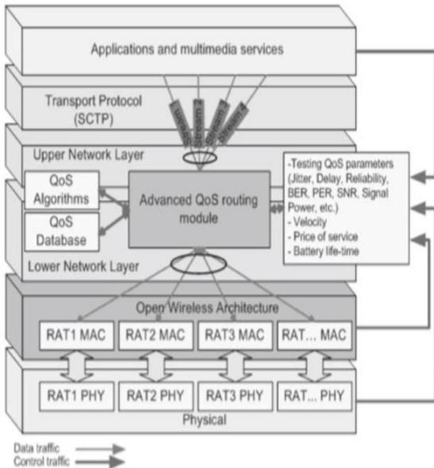
Figure 4. Advanced mobile terminal model [10].
