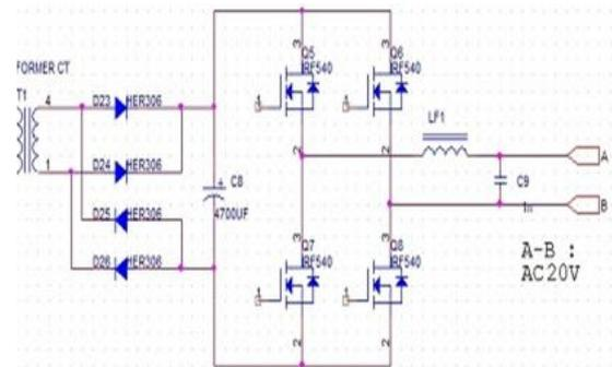
Fig 5. FET inverter circuit
