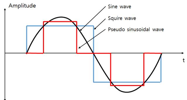
Fig 4. Pseudo sinusoidal wave
