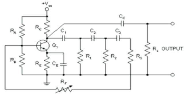
Fig 3. RC phase shift oscillator [11]
