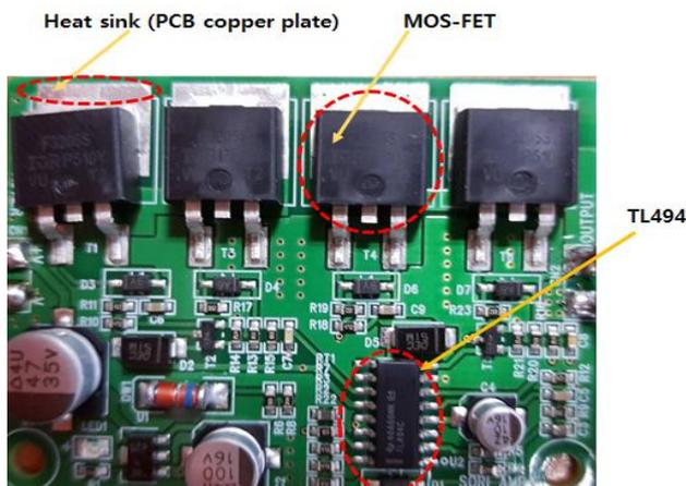
Fig 9. FET pulsed pseudo sinusoidal wave oscillator, amplifier
