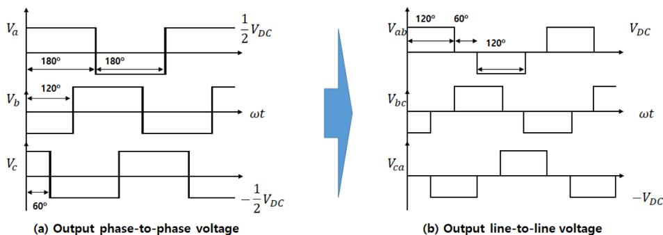
Fig 6. Output of pseudo sinusoidal wave by FET inverter
