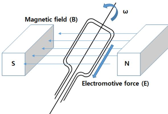
Fig 2. Principles of AC generator [10]
