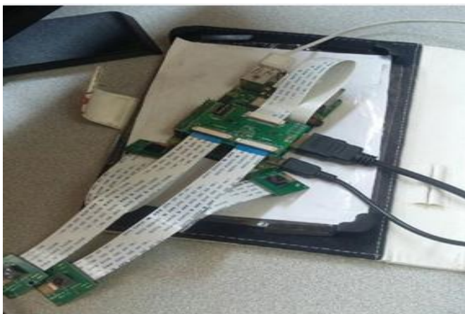
Fig. 2 Multi-adapter assembling with four cameras
