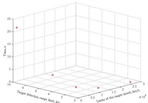
**Fig. 1.** Dependence of the maximum detection range on speed for different numerology values
