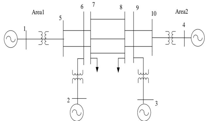
**Fig. 5:** Single line diagram of 4-machine 2-area system.
