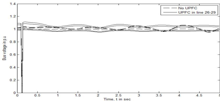
**Fig. 12:** Plot of terminal voltages at buses 26, 27, 28, 29 for a 3-phase fault at bus no. 26
