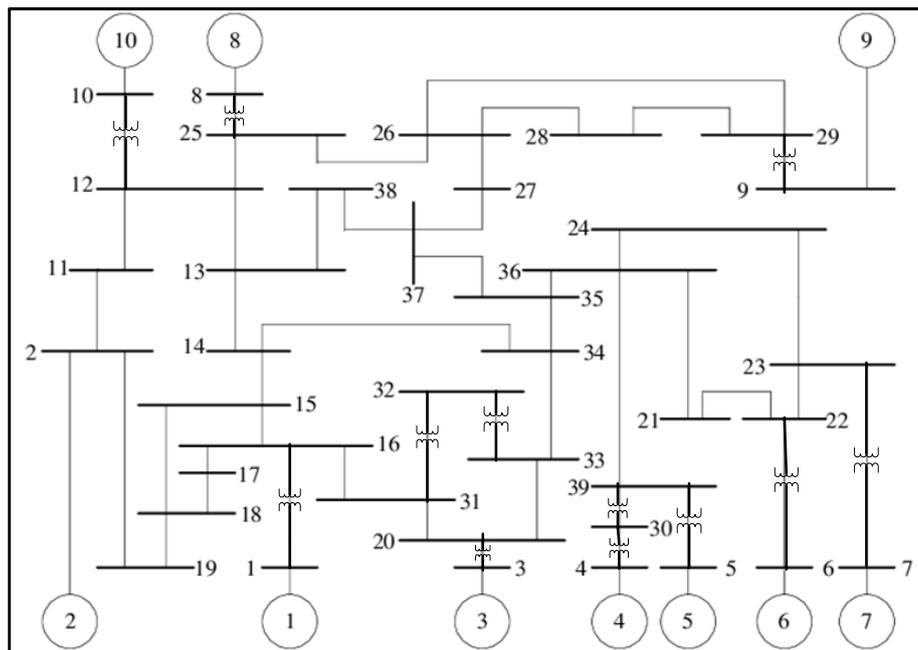
**Fig. 9:** Single line diagram of 10-machine 39-bus New England system.
