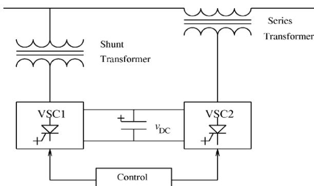
Fig. 1. Unified power flow controller.
