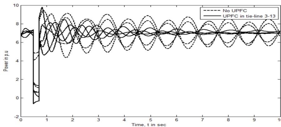
**Fig 8:** Plot of real power of generators 1-4 for a 3-phase fault at bus no. 7.
