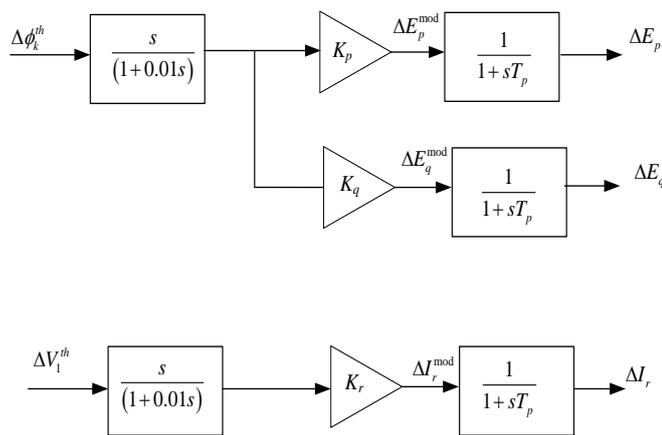
**Fig. 4:** Block diagram of UPFC with supplementary modulation controllers
