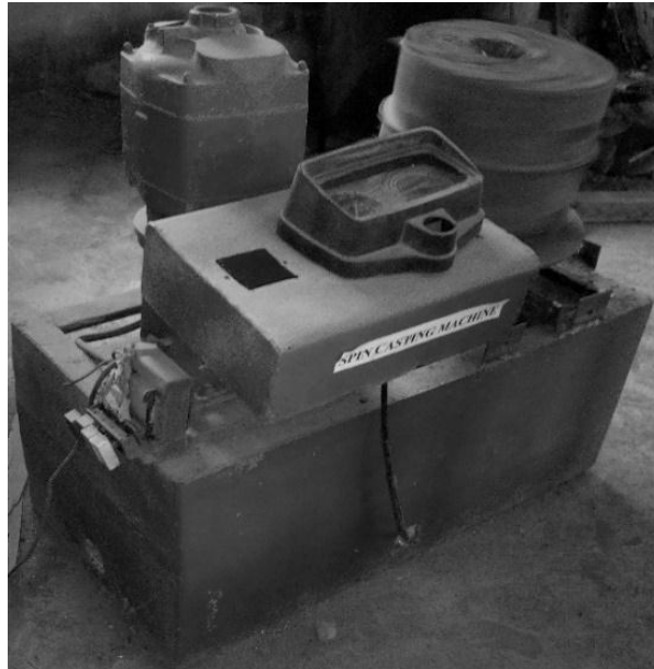
Figure 1 Centrifugal casting setup
