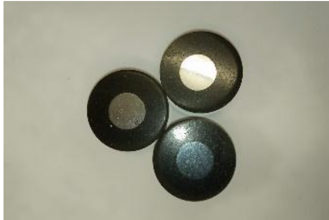
Figure 2. Mounted FGM samples prepared for metallographic analysis
