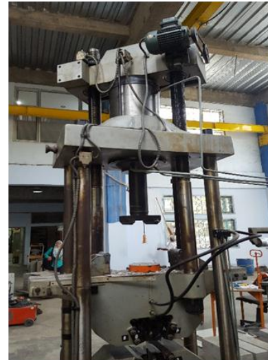
Fig 3. Universal Testing Machine with LVDT and Data Logger
