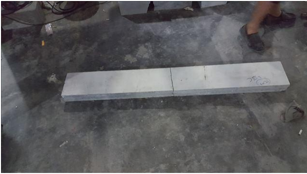
Fig 6. Crack pattern of collapsed beam specimen
