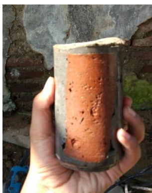
Fig 17. Core Drill specimen
