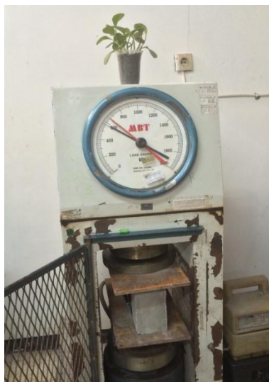
Fig 8. Set up specimen and Compressive Strength Test Machine
