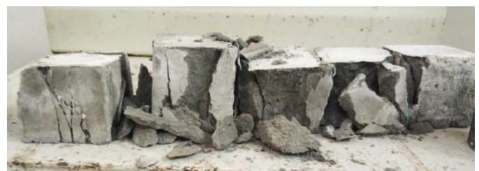
Fig 6. Broken mortar specimens after compressive test
