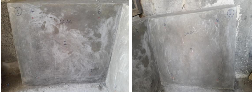
Fig 9. Marking of points of shooting at the surface couple of simple shear walls
