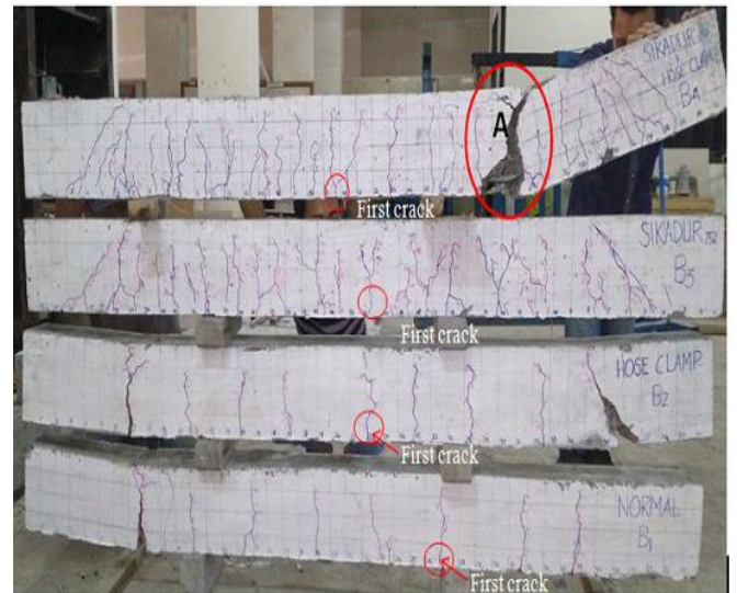
Fig. 9. Crack patterns and fracture behavior of bamboo reinforced concrete beams specimens
