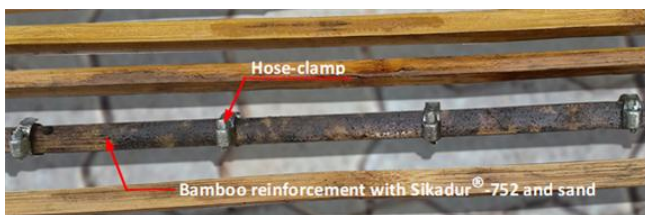
Fig. 2. Treatment of bamboo reinforcement with Sikadur ® -752 and sand
