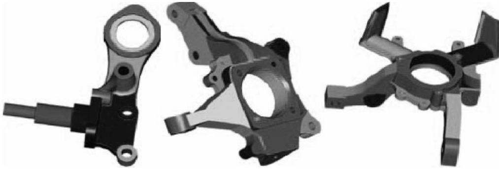
Fig. 1: From left to right the digitized models of the forged steel, cast aluminium and cast iron steering knuckles.
