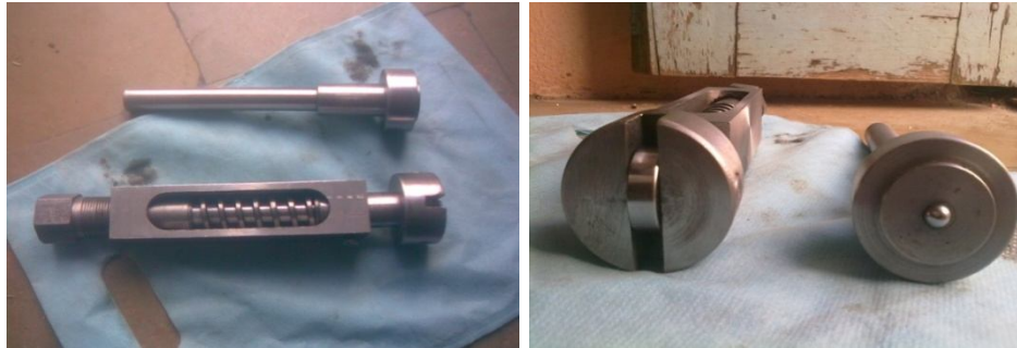
Figure 1: Ball burnishing adapter with roller burnishing interchanging adapter type tool.
