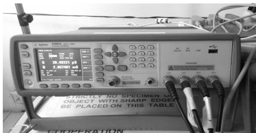
Fig. 1: LCR meter used for damage detection.
