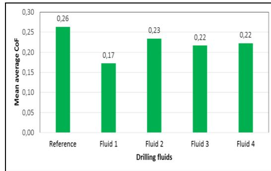
**Figure 8:** Average friction coefficients of the three temperatures data
