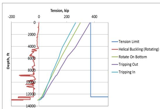
**Figure 11:** Maximum length drilling with the reference fluid without exceeding the tensile limit
