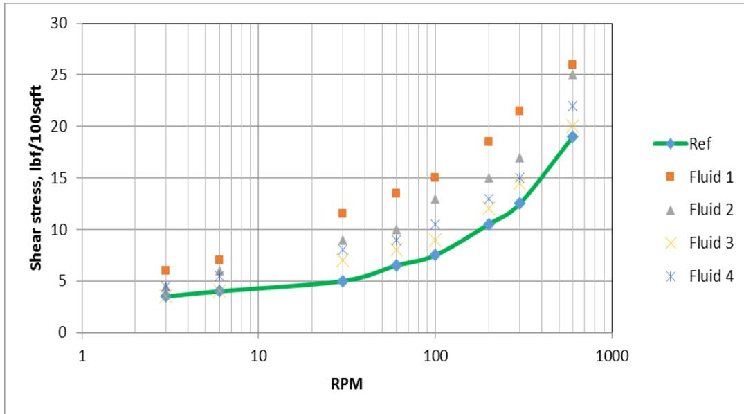
**Figure 3:** Viscometer measurement of test matrix –Table 1.- MoS<sub>2</sub>
