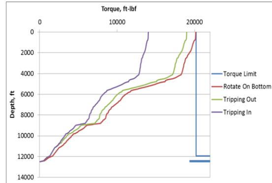
**Figure 10:** Maximum length drilling with the 0.2gm MoS<sub>2</sub> Nano powder treated fluid
