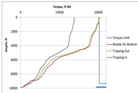
**Figure 9:** Maximum length drilling with the reference fluid without exceeding the torque limit
