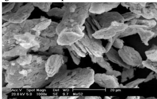
**Figure 1:** SEM analysis of MoS<sub>2</sub> particles
