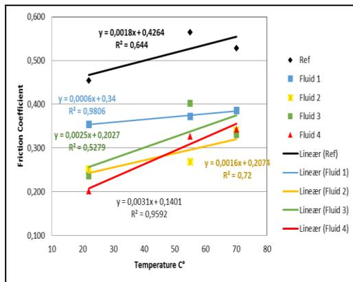
**Figure 5:** MoS<sub>2</sub> treated and reference drilling fluids average friction coefficients
