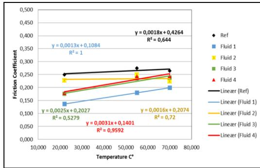
**Figure 7:** Graphene treated and reference drilling fluids average friction coefficients
