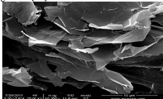
**Figure 2:** SEM analysis of Graphene
