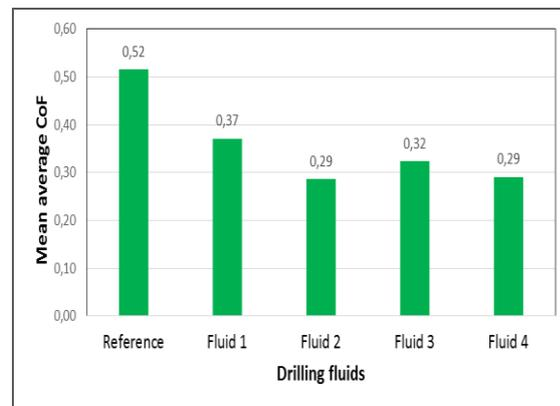
**Figure 6:** Average friction coefficients of the three temperature data
