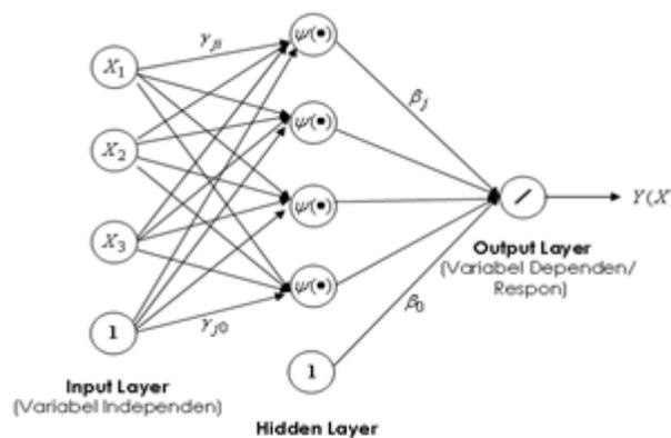
Figure 1: MLP Architecture with single hidden layer, three input units
