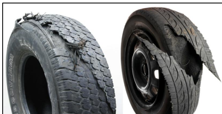
Figure 1 Sample of tyre blowout due to tread separation
