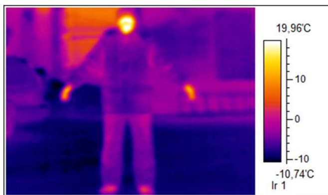
Fig. 15. Thermal imaging test of protective jacket experimental sample
