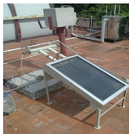
Figure 4. Image of the thermosyphon solar water heater experimental set-up.
