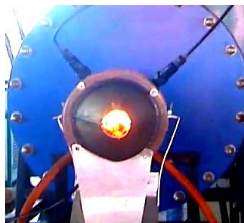
Fig. 11. Sustained combustion with rich mixture of fuel
