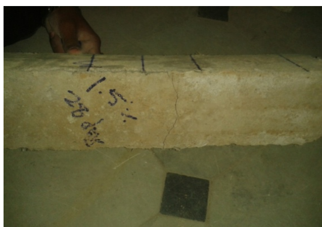
Volume fractions-1.5% Polypropylene specimen after testing
