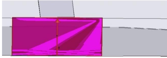
Figure 3: LumpedPort Excitation Shown In Color Portion
