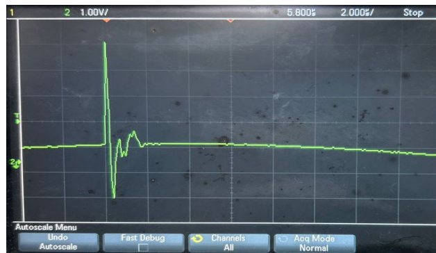
Figure 10. Output waveform of the 0.5 mm Rogowski Coil during pulse testing
