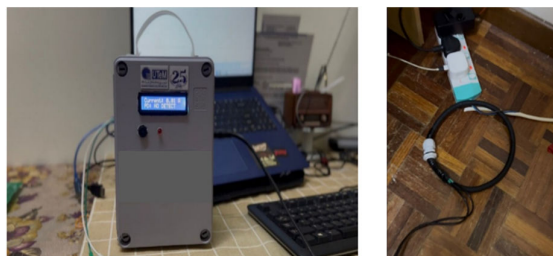
Figure 7. Hardware testing setup with Rogowski coil placed around the extension cable
