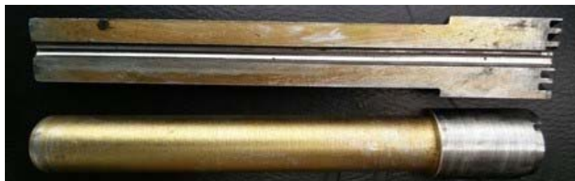
Fig.11. Fabrication of Hollow Cylindrical Plunger
