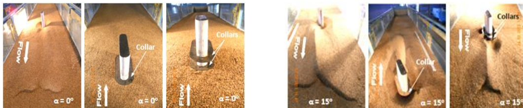
Figure 6: Photographs showing placement of collars around pier and scour pattern formed after the experiment.
