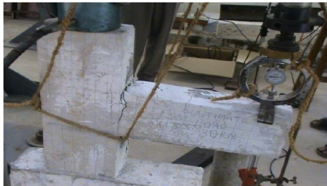
Figure 2.2: Failure due to Ultimate Load for Control Specimen.
