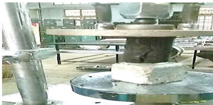
Fig. 4: Testing of Peat Soil Sample in UCC Machine
