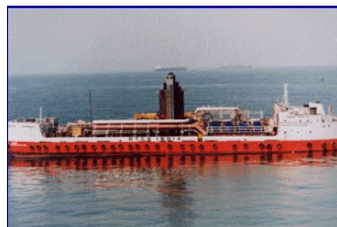
Fig. 6: Rankine Cycle based OTEC power plant.
