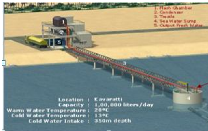
Fig. 3: Low temperature desalination plant.
