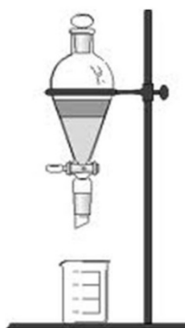
Fig. 5: Neem biodiesel and glycerin separation setup.
