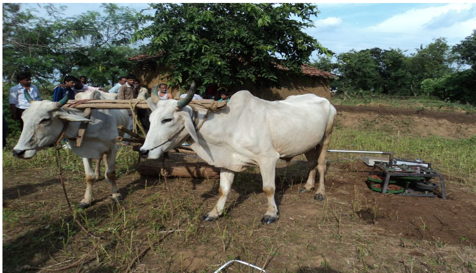
Fig. 3: Animal powered mechanical device for home lighting system.
