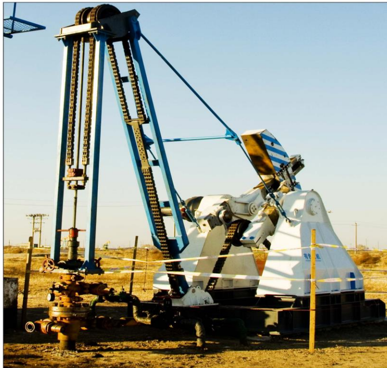
Fig.6 Field test of the new pumping unit
