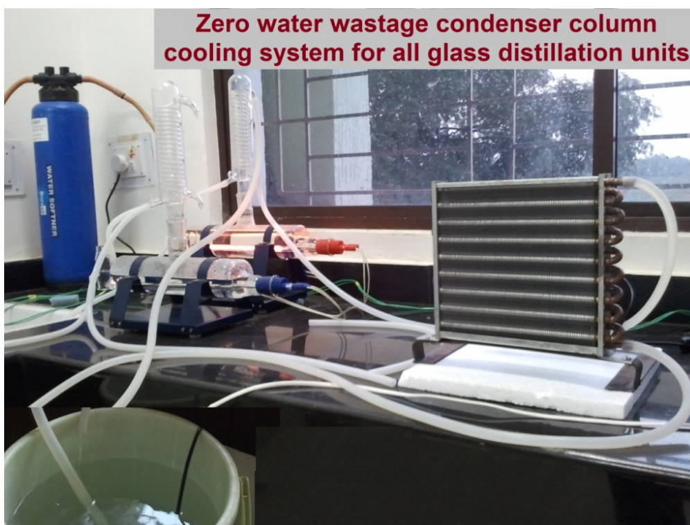
Plate1: Zero water wastage condenser column cooling system fitted to all glass distillation unit at our laboratory
