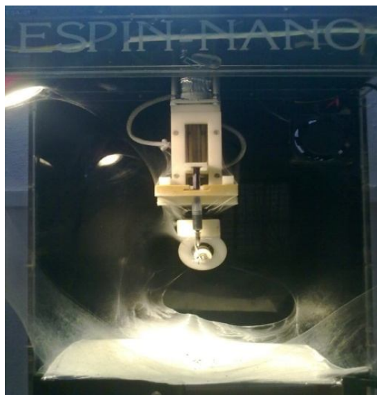
Figure 1: Picture of the electrospin apparatus with the nanofibers formed at the bottom collected in a planar sheet.
