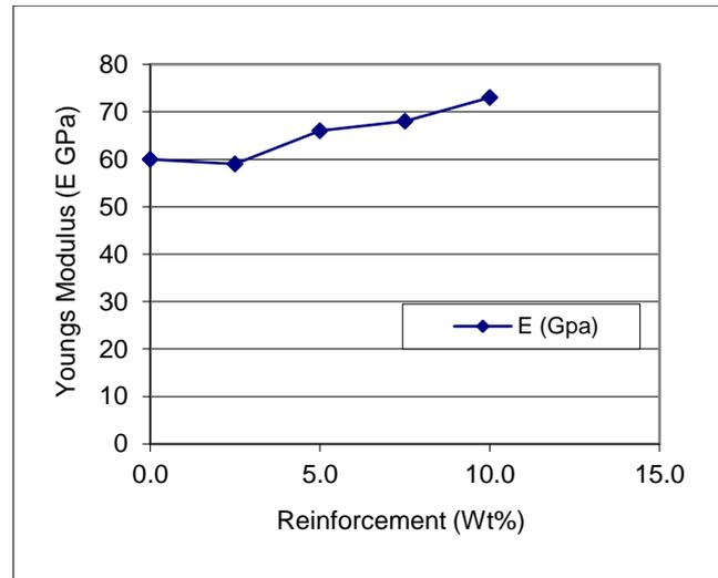
**Fig. 3.** Young modulus versus volume fraction of reinforcement
