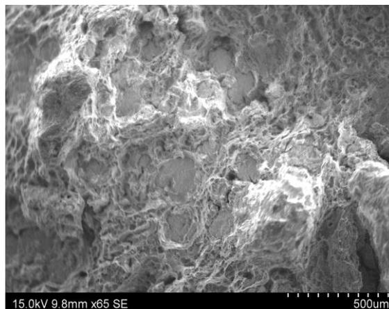
**Fig. 8.** Fractograph of 10% Al<sub>2</sub>O<sub>3</sub> red mud particulates reinforced hybrid metal matrix composite after tensile testing.
