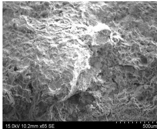
**Fig. 7.** Fractograph of 7.5% Al<sub>2</sub>O<sub>3</sub> red mud particulates reinforced hybrid metal matrix composite after tensile testing.
