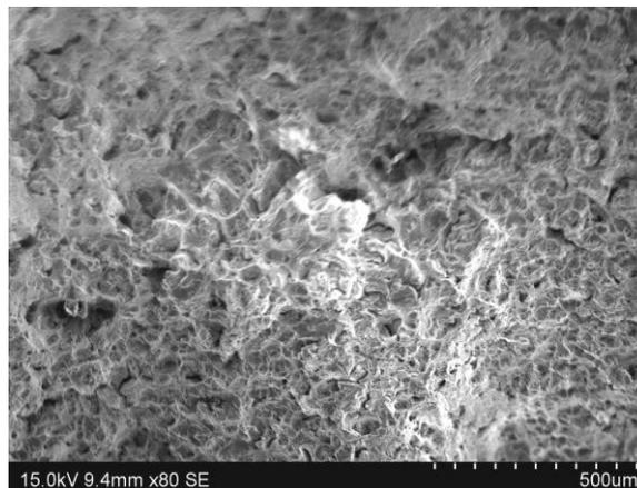
**Fig. 6.** Fractograph of 5.0% Al<sub>2</sub>O<sub>3</sub> red mud particulates reinforced hybrid metal matrix composite after tensile testing.
