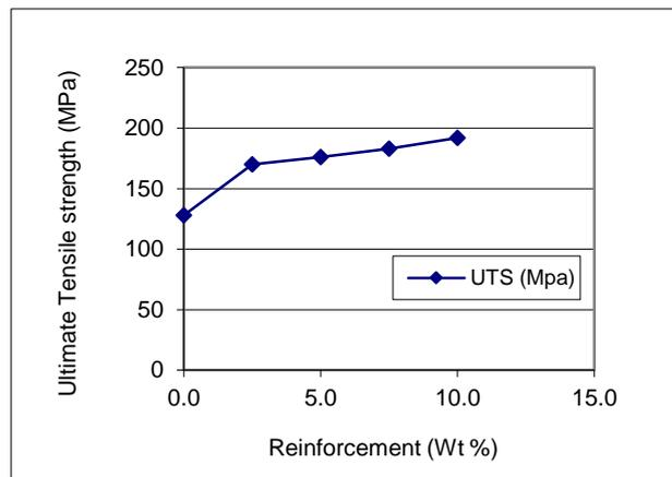
**Fig. 2.** Tensile strength versus volume fraction of Al<sub>2</sub>O<sub>3</sub> and red mud
