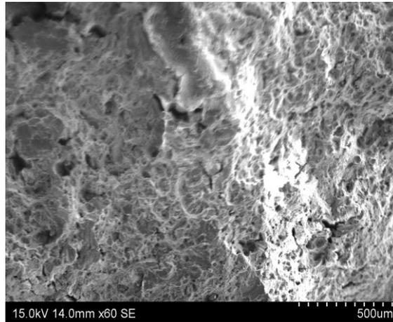
**Fig. 5.** Fractograph of 2.5% Al<sub>2</sub>O<sub>3</sub> red mud particulates reinforced hybrid metal matrix composite after tensile testing.
