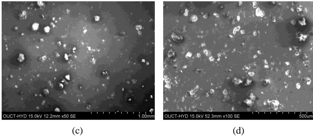
**Fig. 1.** SEM micrograph of Al<sub>2</sub>O<sub>3</sub> Red mud particle reinforced composite (a) 2.5% (b) 5.0% (c) 7.5% (d) 10.0% reinforcement.
