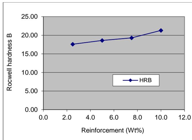
**Fig. 4.** Hardness versus Reinforcement volume fraction
