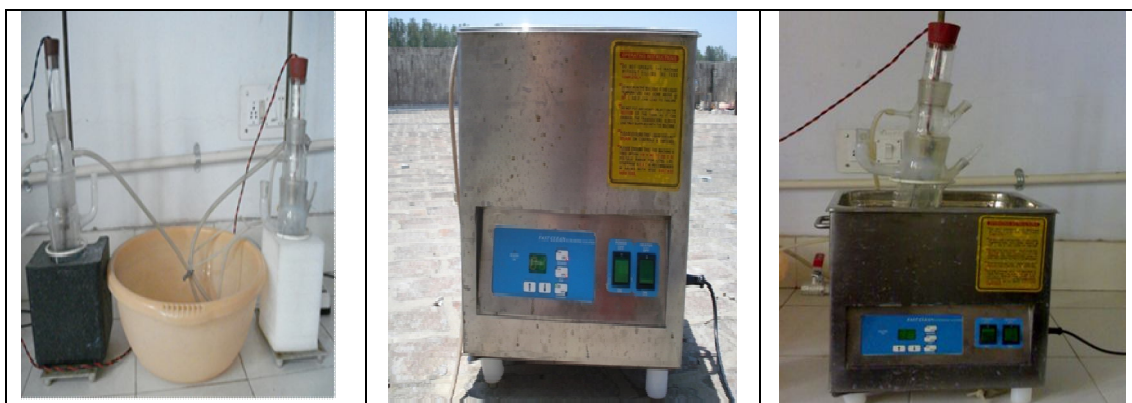
Figure 1. Photocatalytic reactor, sonicator bath and Sonophotocatalytic reactor
