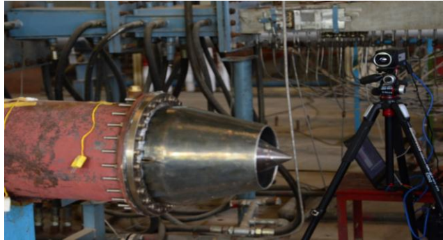
Fig 7: Picture of test rig with Thermal Imaging Camera
