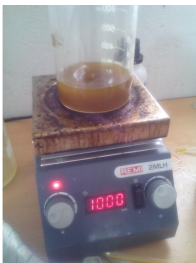
Figure 1 Magnetic stirrer with the neem oil
