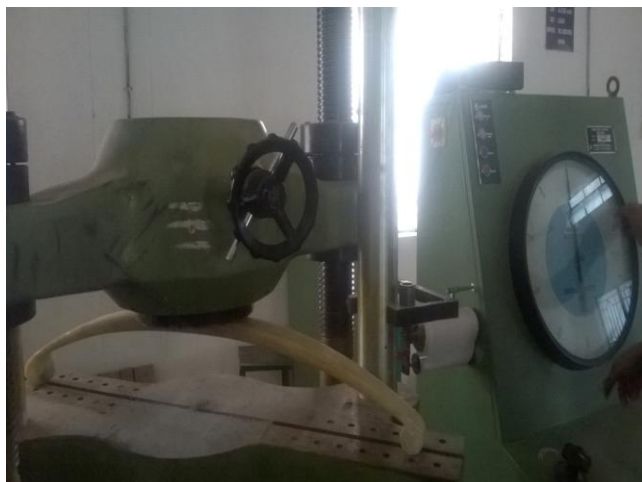
Fig 5.1 Testing of the composite leaf spring
