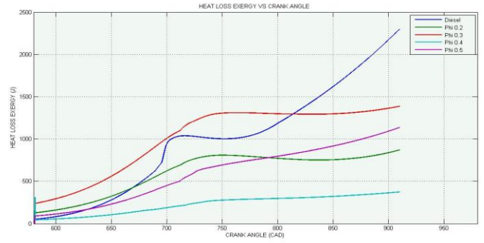
Fig 9. For various Equivalence Ratio of CNG Heat Loss Exergy with crank angle
