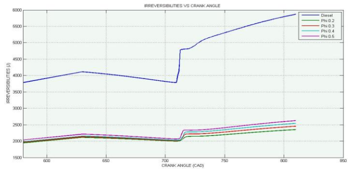
Fig 10. Irreversibilities for varies equivalence ratio of CNG and Diesel
