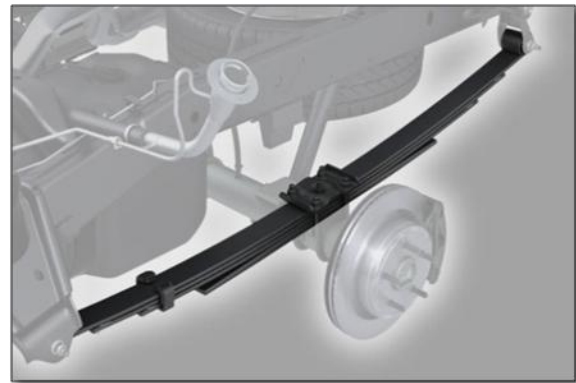
Fig.1.4 Leaf Spring – Automotive
